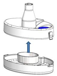
c. Unthread and remove fill cap from vaporizer lid, and drain remaining liquid into a sink.
