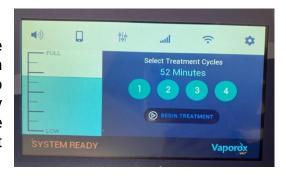
Once the control panel is turned on via the power switch on the left side of the control panel, a Select Treatment Cycles screen is displayed on the touchscreen with the default treatment settings.
