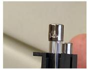
3. Insert the fuse holder into the power module at the back of the VHT-200.
